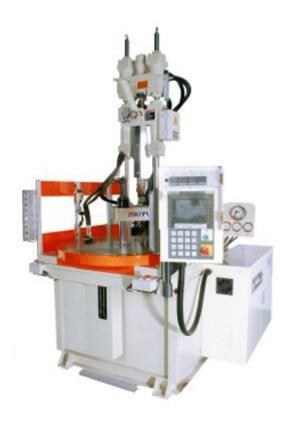
Clamping Force: 10 - 500 ton/ Injection Capacity: 0.5 - 50 oz
